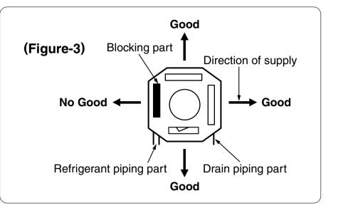
(Figure 3 shows a view seen from the drain pan.)
