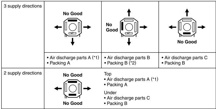
\*1: For the models MMU-AP0091H~AP0151H, use the air discharge parts A (410mm in length) which is prepared by cutting off 60mm. \*2: Use packing B (410mm in length) which is prepared by cutting off 50mm.
