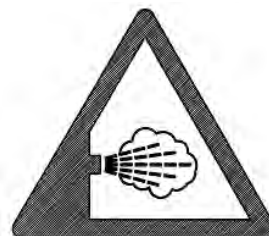
Warning - safety valves' vents
