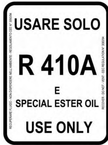
Identification of the refrigerant - External door
