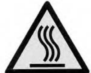
Warning - high-temperature zones Adjacent to hot pipes or components
