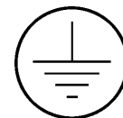
Grounding connection - On the electrical board, adjacent to the connection
