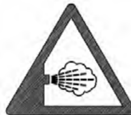
Warning - safety valves' vents
