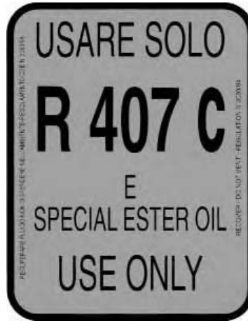
Identification of the refrigerant - External door
