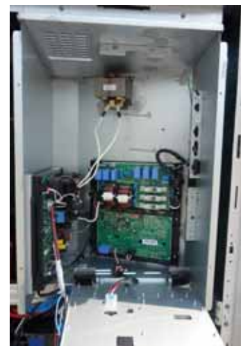
► Separate double layer structure of C/Box after remove 3 screws and connector.
