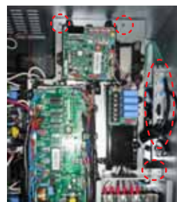
► Separate double layer structure of C/Box after remove 3 screws and connector.
